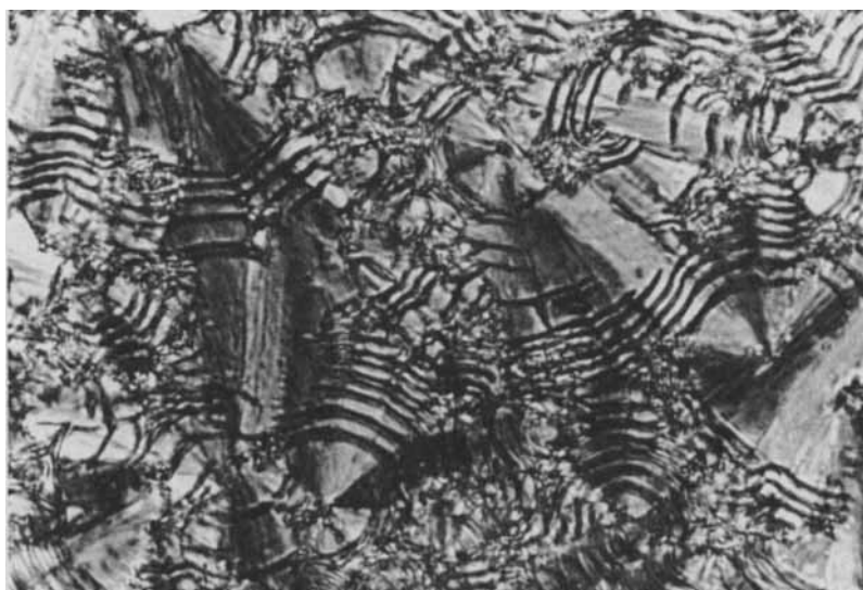
FIGURE 4 A texture of Sm C* DOBAMBC non-oriented sample 50\text{ }\mu\text{m} thick just after d.c. field E = 3\text{ kV/cm} has been applied. Remaining dechiralization lines are seen. The area of the figure is (0,37 \times 0,25)\text{ mm}^2 .
