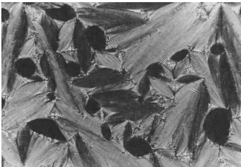
FIGURE 3 A fan-shaped texture with dechiralization lines in DOBAMBC non-oriented sample 30\text{ }\mu\text{m} thick in Sm C* phase as seen between crossed polarizers. The black areas are air bubbles. The area of the figure is (0,37 \times 0,25)\text{ mm}^2 .
